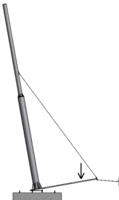
Figure 12 – Catching the gin-pole
