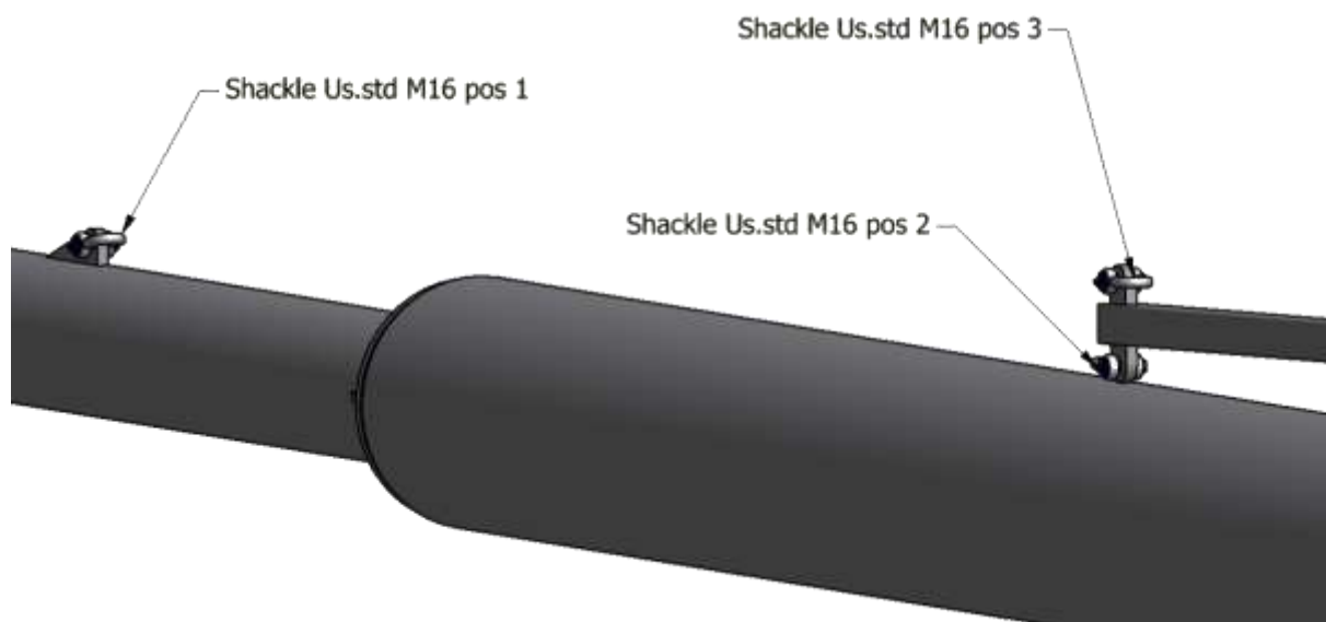
Figure 10 – Placing the gin-pole cables
