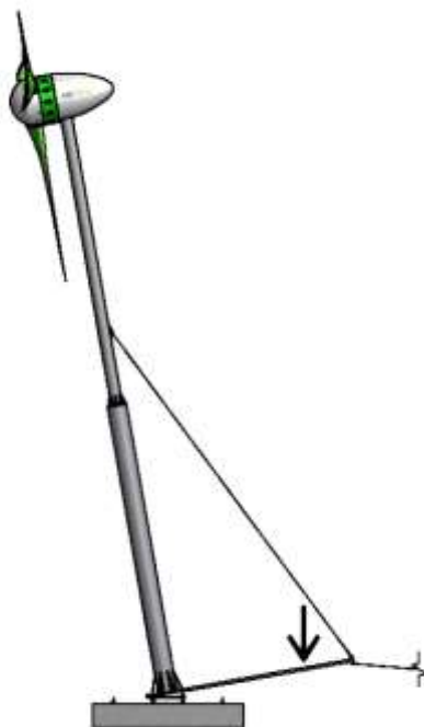
Figure 22 – Catching the gin-pole
